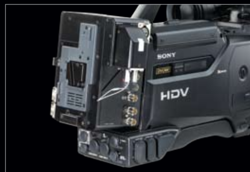
The rear-attached NIPROS PS-470L camera adapter easily converts the HVR-S270U shoulder mount HDV camcorder for studio applications.
